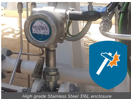
High grade Stainless Steel 316L enclosure
