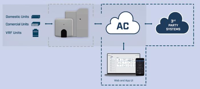
AC Cloud Control is an HVAC IoT solution created by Intesis for building and facility management. A cloud-based remote-control system, that allows comfortable and intuitive control of air conditioners and heat pumps from a smartphone, tablet, smart watch or from a simple internet browser.
